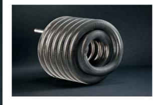
Stainless steel finned coils are produced from Laserfin<sup>®</sup> tubes. The excellent laser-welded connection between tube and strip enables an unproblematic bending and coiling of the finned tube.
